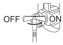
Figure 43. On-board Water Tank ON/OFF Valve
